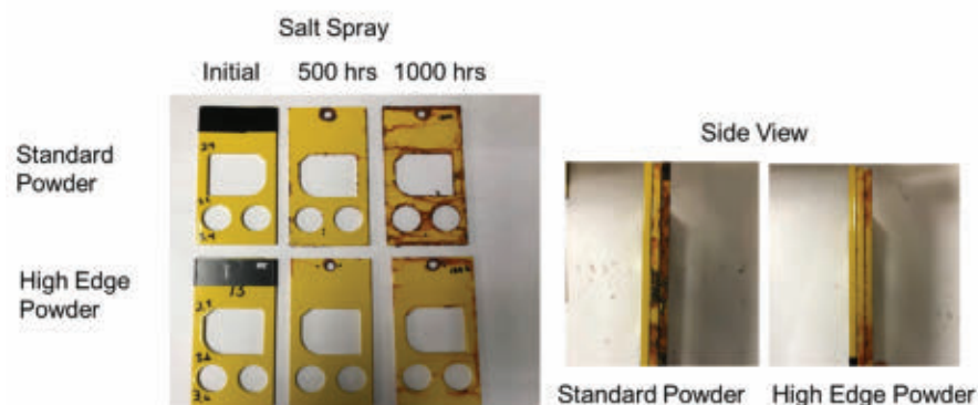
Figure 3: Salt spray results for a standard powder formulation and one modified for edge-protection. Significant performance improvement is evident in the high-edge formulation.
